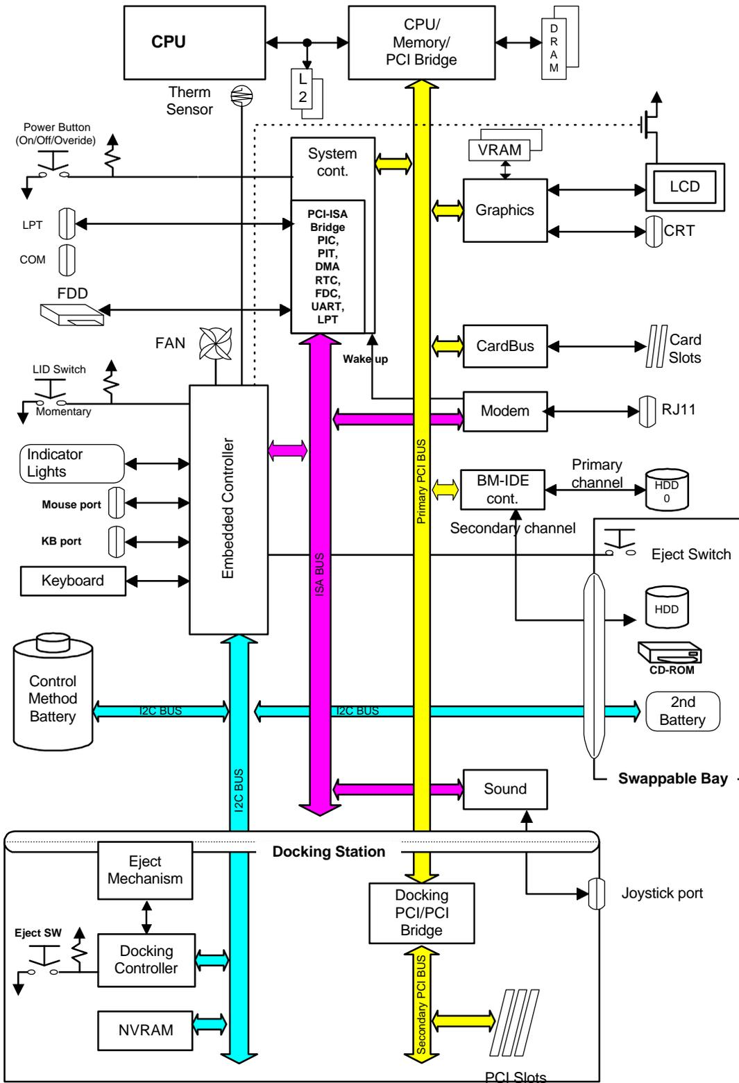
Figure 2-1 Mobile Concept Machine Hardware Block Diagram
