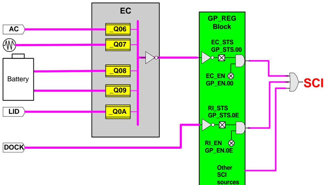
Note that in the preceding block diagram, a non-embedded controller event, the docking event, is shown tied to `GP_STS.0E`; this is a general-purpose event. AC adapter, thermistor, battery, and lid events could all be handled as general-purpose events, also. Using an embedded controller on a platform is totally optional. Some advantages of using an embedded controller are:
