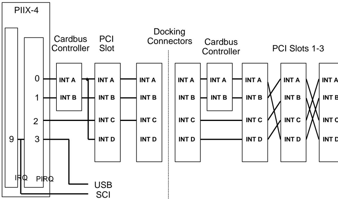
The interrupt structure to the left of the line labeled “Docking Connectors” in the diagram can be modeled as a PCI interrupt routing table using ASL code as shown below.
