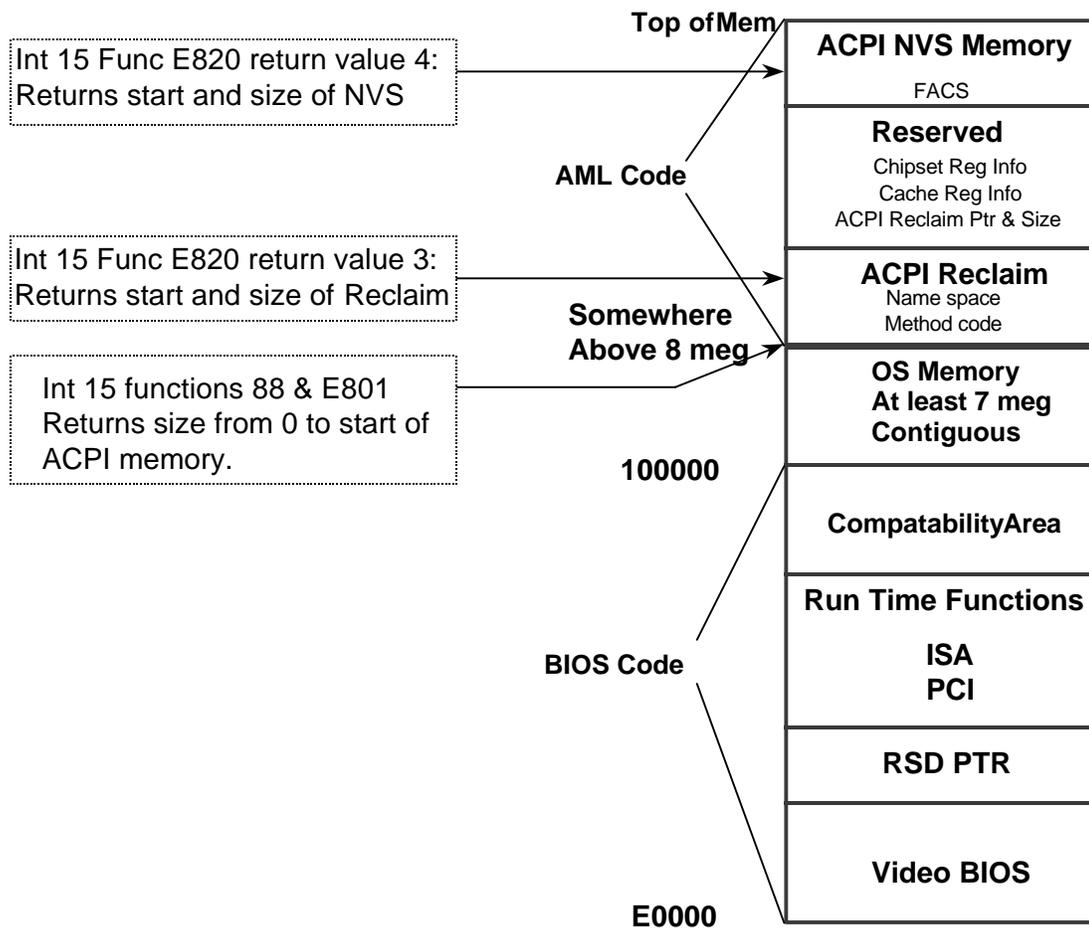
The annotations on the above illustration point out the DOS Int 15H functions the BIOS can use determine the size and location of various types of memory:
