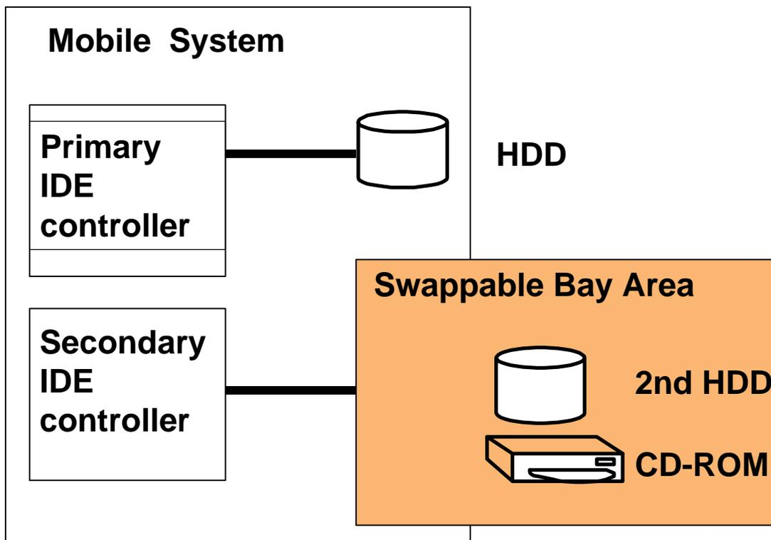
When a second HDD device is inserted in the Bay, two IDE controllers and two IDE HDD devices are active. Which IDE controller controls the primary channel and which IDE controller controls the secondary channel is encoded in the `_ADR` object under each IDE controller's Device object in the ACPI name space, using the following convention:
